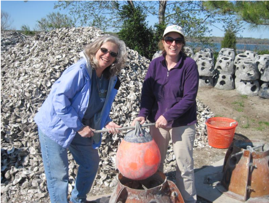
Patty Maloney and Christina Woodson making "reef balls" at VIMS waterside as part of the Chesapeake Bay Foundation's oyster restoration project."
